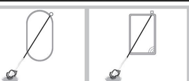
GB First, lay down all hose sections on the ground under sunlight for about an hour to remove hose memory. Second, measure your pool to figure out total length of hose needed for cleaner operation. Total length of hose after assembly should be half to one hose section length longer than the length measured from pool skimmer / dedicated suction line to the farthest point in the pool.
