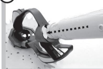
GB Insert the diaphragm chamber "C" into the support "A". Align the side pins on diaphragm chamber with the notches on the support "A", and continue to insert the chamber into the chamfer of the support. Follow the arrow direction of marking "F" and turn the chamber until it stops.
